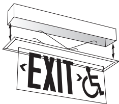
Trim and faceplate mount into backbox for quick and easy installation.
